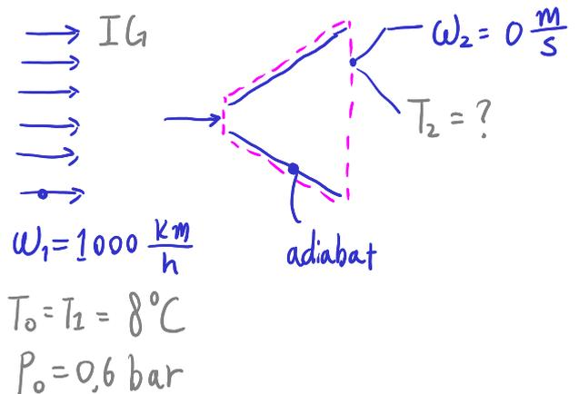
$$\frac{dE}{dt} = \dot{m}_1 \left( h_1 + \frac{w_1^2}{2} + pE_1 \right) - \dot{m}_2 \left( h_2 + \frac{w_2^2}{2} + pE_2 \right) + \dot{Q} - \dot{W}$$
